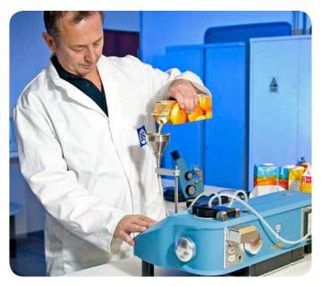
Fig. 8: The Pro-Juice refractometer pre-conditions orange juice samples so that lines can run just above the lower threshold of product filling specification providing optimum yield from concentrates and thus helping to improve profitability from reduced waste or "over Brixing."
